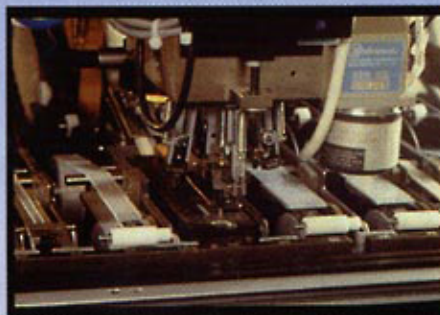
Automatic placement of the jumper onto the IMS surface mount pads. The terminal strip is advanced into the shear station (left) where the jumper is singulated and positioned for pickup by the placement head. It is then placed (right) onto the paste-coated solder pad.
