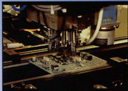
Automatic placement of the jumper onto the IMS surface mount pads. The terminal strip is advanced into the shear station (left) where the jumper is singulated and positioned for pickup by the placement head. It is then placed (right) onto the paste-coated solder pad.
