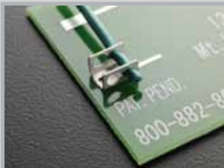
View of part after wire termination
